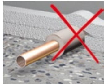
Incorrect floor design: Tube projects into the insulation
