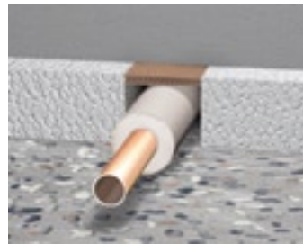
Proper installation of WICU® tubes on raw concrete floors by creating an even surface and adequate gaps for expansion movements
