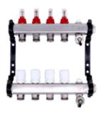
Manifold in AISI 304L stainless steel with terminal group, manual vents and flow meters. Flow rate: from 1 l/min to 5 l/min
